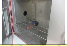
High Temperature/ Humidity Test Low Temperature Test
